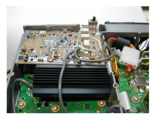
29.) Lay the flat-ribbon connector over the middle wall of the transceiver so that it does not disturb or damage it.
